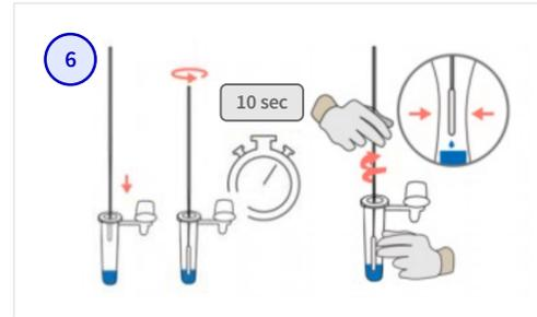
Place the swab in the extraction tube. Rotate the swab for about 10 seconds, Rotate the swab against the extraction tube, pressing the head of the swab against the inside of the tube while squeezing the sides of the tube to release as much liquid as possible from the swab.
