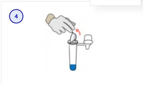
Peel off aluminium foil seal from the top of the extraction tube containing the extraction buffer.
