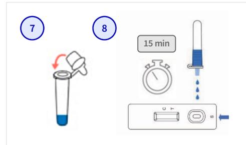
Mix thoroughly by flicking the bottom of the tube. Place 3 drops of the sample vertically into the sample window of the test. Read the result after 15 minutes.
