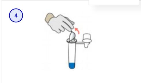
Peel off aluminium foil seal from the top of the extraction tube containing the extraction buffer.
